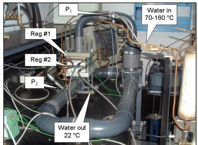
Figure 6 Experimental setup of the two stage engine.
